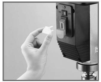
Fig. 4. Remove Switch Safety Key when not in use.
